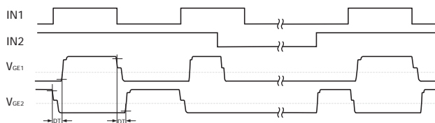
Figure 9. Transmission logic in half-bridge mode
